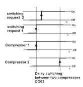
CO04 Off delay time between compressor or stage valve.
