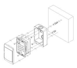
The temperature range allowed for correct operation is --10÷60°C. Avoid places subject to strong vibrations, corrosive gases, excessive dirt or humidity. The same recommendations apply to probes. Let air circulate by the cooling holes.
