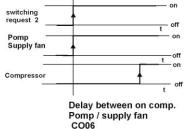
**C007** "Water pump / air supply fan" switch off delay time after compressor deactivating.
