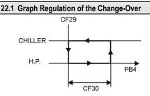
When the temperature value is within the **CF30** range, the changeover is allowed only though keyboard.
