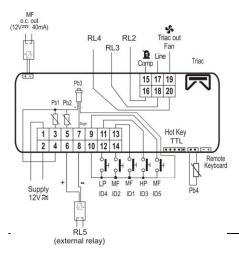
MF ID1, MF ID2, MF ID5 = multifunction digital inputs ID3 = high pressure digital input ID4 = low pressure digital input RL1 = compressor relay MF RL2, MF RL3, MF RL4 = multifunction relays RL5 = output for multifunction external relay Triac out fan = output for condenser fan Pb1, Pb2, Pb4 = NTC probe or digital input Pb3 = ratiometric pressure trasducer MF o.c. out = multifunction open collector output (for external relay)
